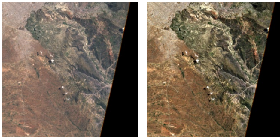
Figure 2-12 – Left: Level 1C Input, Bands 2-4; right: Level 2A Output, Bands 2-4, RGB composite images, scene from La Paz on
