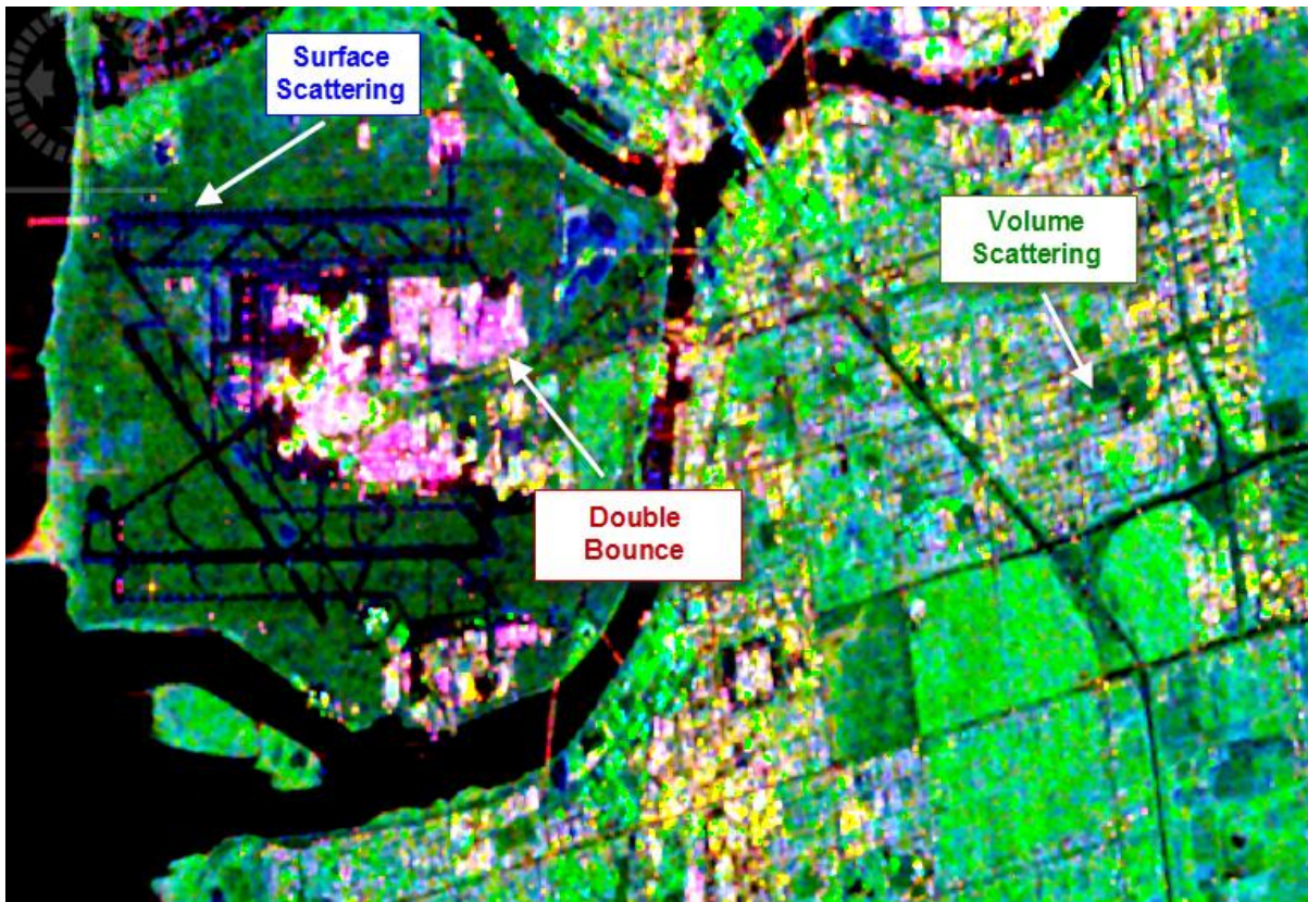
Figure 13: Scattering mechanisms in the Freeman-Durden Decomposition
