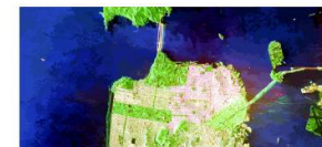
Fig. 1.9. Radarimetric RGB image over San Francisco (USA) where the colour code is: S_H , blue, S_V , red and S_H , green. Filtered image with the BPT speckle filter.
