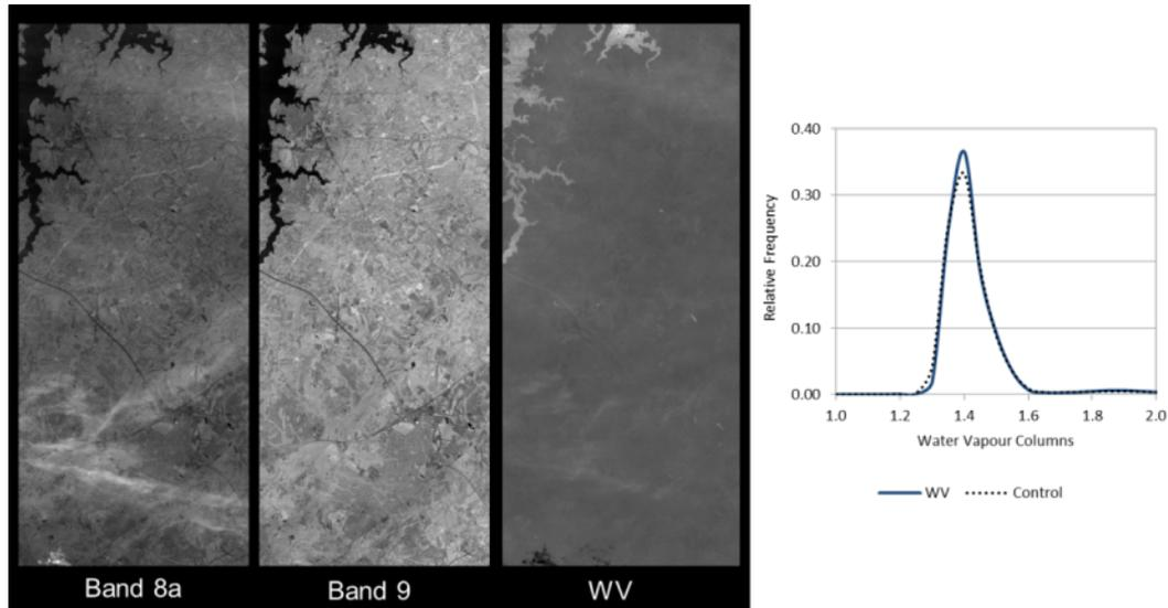
**Figure 3-10 – WV Retrieval using Bands 8a and 9**
