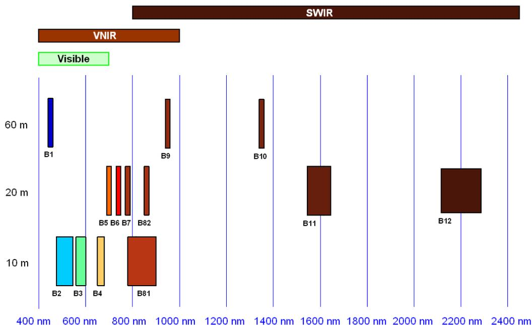
Figure 3-1 – Sentinel-2 Spectral Bands and Resolutions
