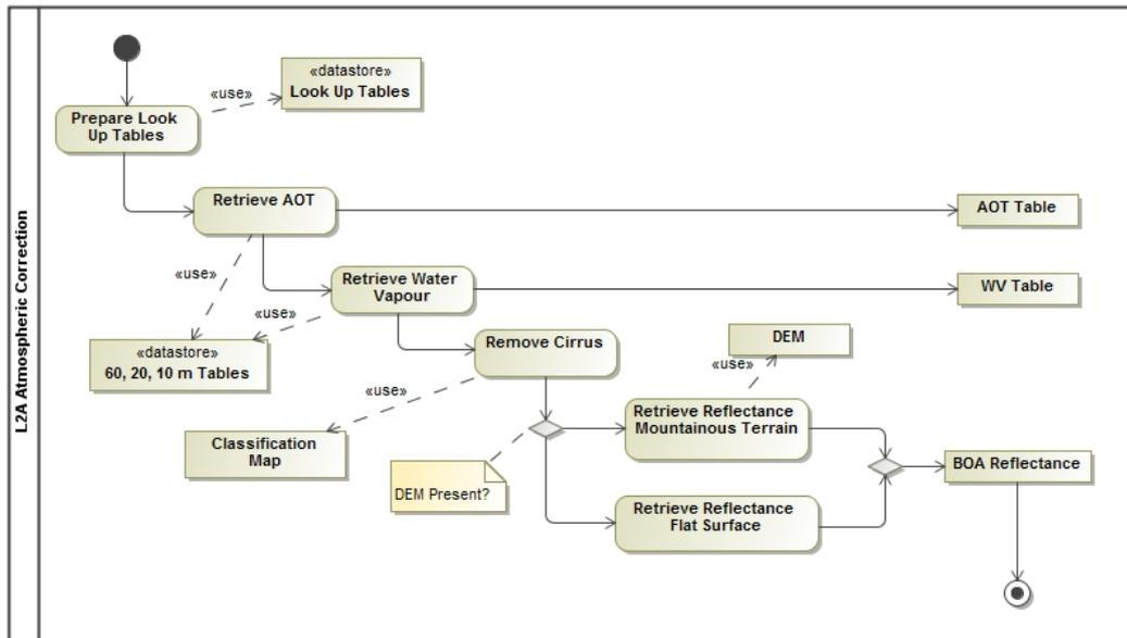
**Figure 3-8 – Atmospheric Correction, Processing Flow**
