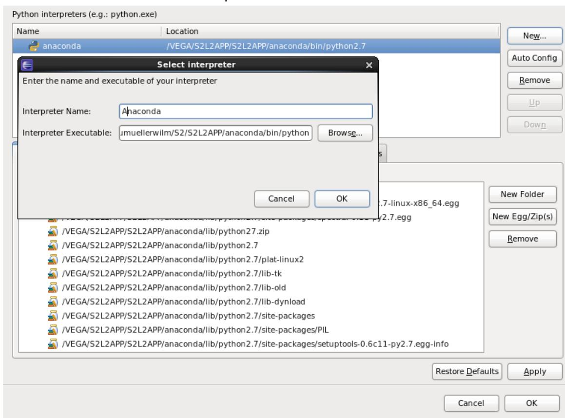
**Figure 4-4 – Configuration of Python interpreter within Eclipse II**
