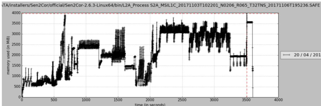
Figure 2-15 Memory Consumption during processing
