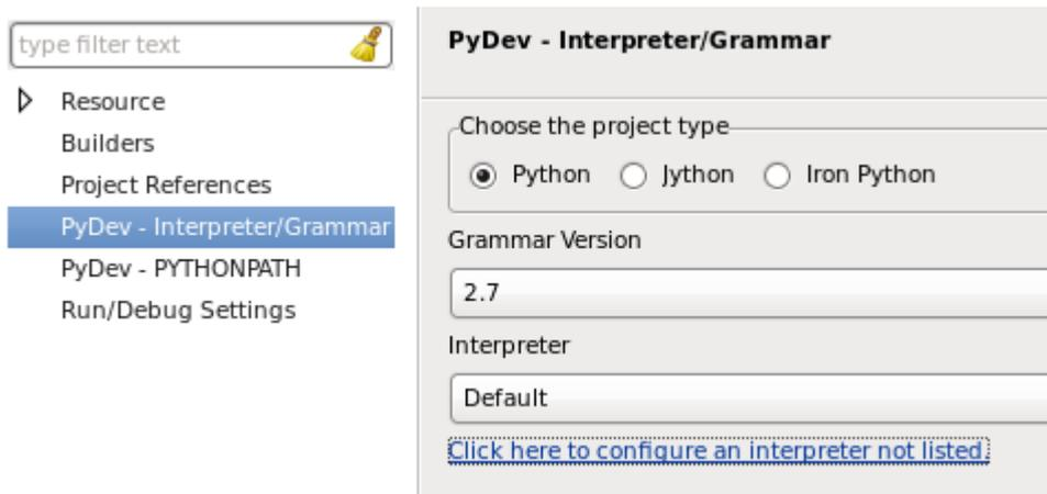
**Figure 4-3 – Configuration of Python interpreter within Eclipse I**
