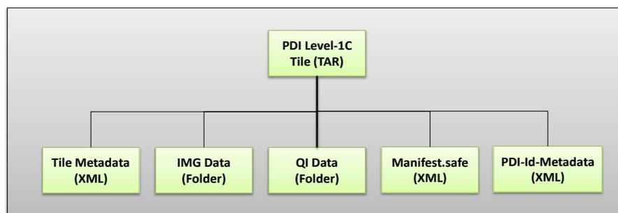
**Figure 3-14 – Filing structure of Level-1C product on tile level**
