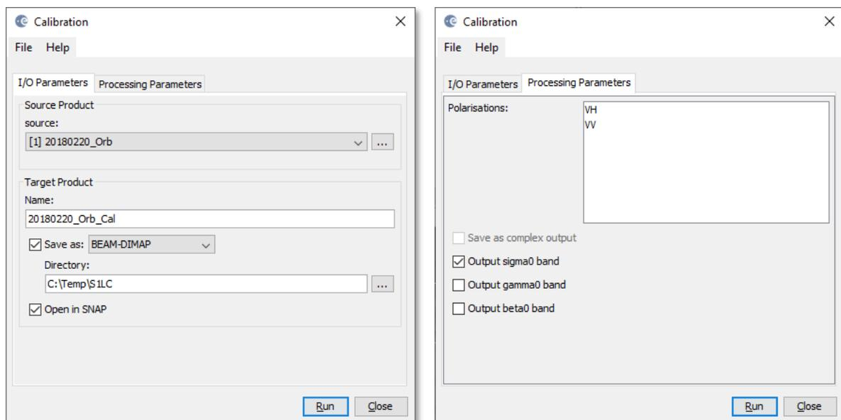
Figure 8: Radiometric Calibration
