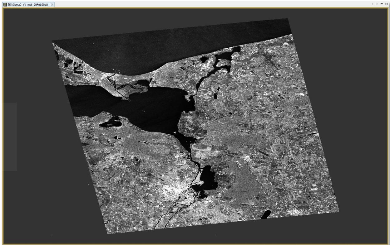
Figure 17: Geocoded image product after Terrain Correction
