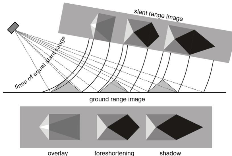
**Figure 15: Geometric distortions in radar images (Braun 2019)**
