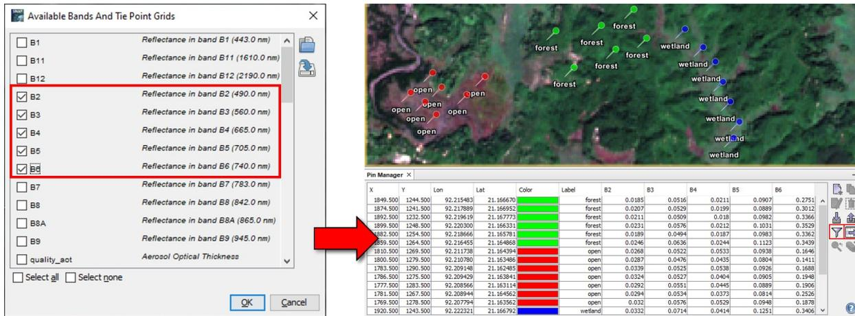
Figure 8: Extraction of pixel values under pins
